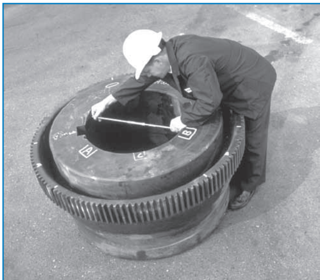
KOP-FLEX service technician inspecting gear coupling
