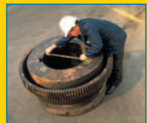
KOP-FLEX service technician inspecting gear coupling
