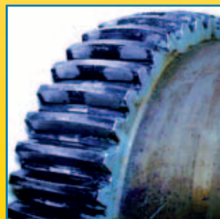
Lapped gearing with blue contact check at 3° 60-70% gear teeth in contact good finish, corrected for carburizing distortion
