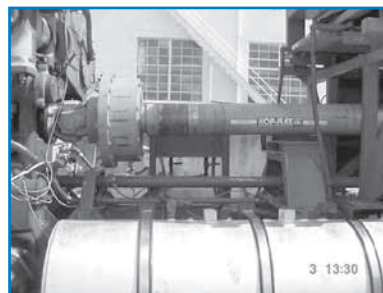
U-Joint with MAX-C® resilient coupling on a truck-mounted pump/transmission system for an oil patch application.
