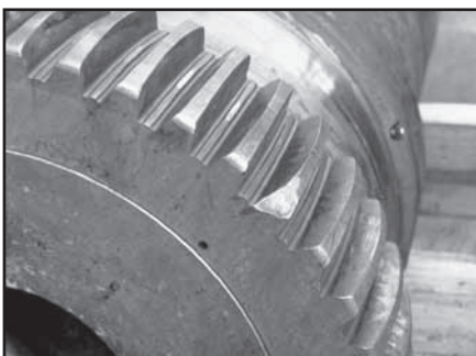
Tooth End Breakage due to over-misalignment
