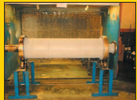
LM 2500 gas turbine coupling after complete refurbishment
