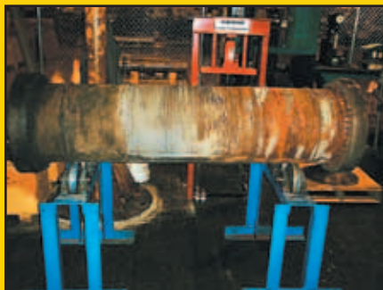
LM 2500 gas turbine coupling before being refurbished
