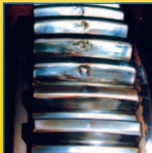
Localized spalling resulting from uncorrected carburized gearing
