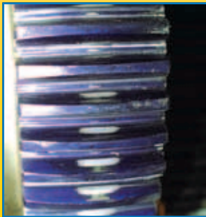
Uncorrected carburized gearing with blue contact check at 3° 20-40% gear teeth in contact
